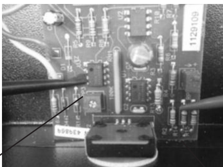
Black Lead to U3 Pin 3 Here Front of Control Drawer Red Lead to R14 Here
