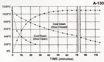
Test Conditions: nominal line voltage, no load in the muffle, control set to 1100°C. Lower temperatures will require approximately the same amount of heating time due to the nature of the control. Setting the control higher than the desired setpoint and then reducing it will shorten the total time.
